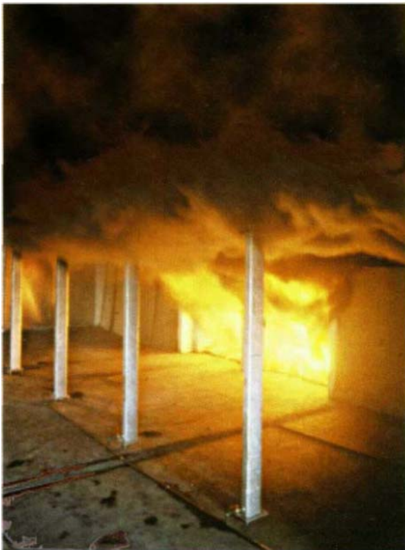
Plate 5 Smoke spreading beneath a balcony
