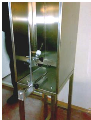
Apparatur i henhold til EN 60332-1-1:2004 (Foto: MARES Engineering Research Electronic Systems, Tyrkia. www.maresteknik.com/up/image/5.png )
