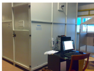
Apparatur i henhold til EN 61034-2:2005 (Foto: MARES Engineering Research Electronic Systems, Tyrkia. www.maresteknik.com/up/image/2.png )
