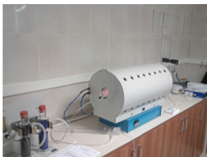
Apparatur i henhold til EN 50267-2-3:1998 (Foto: MARES Engineering Research Electronic Systems, Tyrkia. www.maresteknik.com/up/image/4.png )
