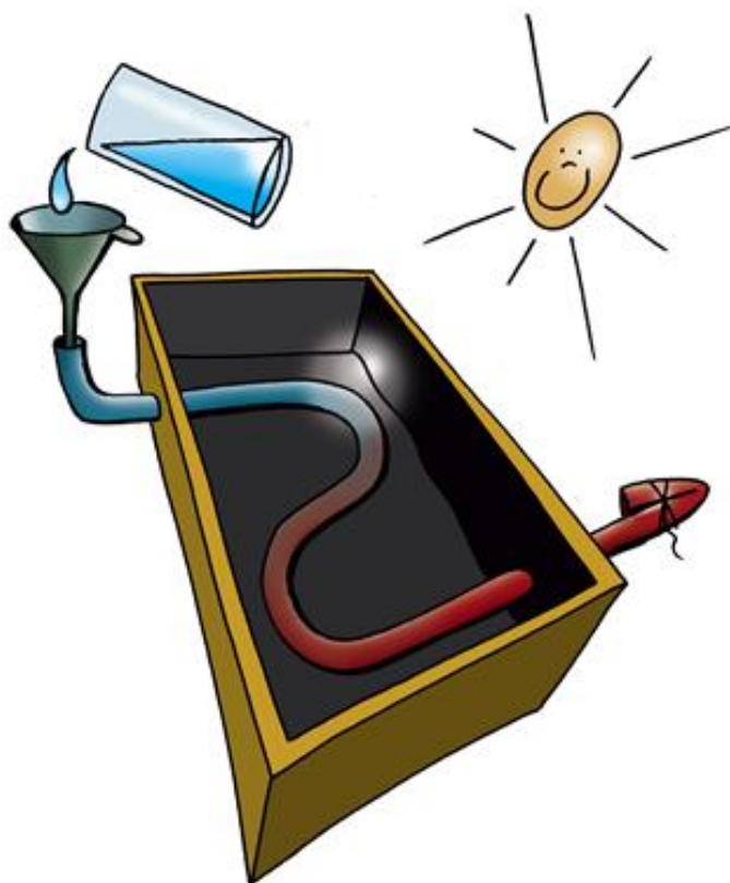
Figur 19. Prinsippskisse for platesolfanger.
